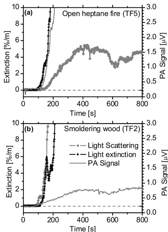
Figure 3: Evolution in time of the scattering, extinction, and absorption (photoacoustic detector) of light during two different test fires. The raw signal in  $\mu\text{V}$  of the PA sensor is shown at the right of the graph. The calibrated signals, including the photoacoustic sensor, are shown to the left of the graph. The left axis is defined in terms of the light extinction sensor. Therefore, the light scattering and photoacoustic signal can at most equal that of the extinction sensor.
