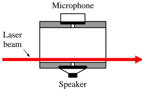
Figure 1: Schematic view of the PA cell
