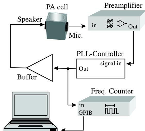
Figure 2: Resonance tracking circuit. The phase of the second azimuthal resonance is continuously monitored by a Phase Locked Loop (PLL). Theoretically, the PLL should lock to the frequency whose phase is equal to zero (i.e. the second azimuthal frequency). The electronics must compensate for the phase shift induced by other factors like the band pass filter of the preamplifier.
